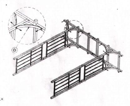
5. Place the fully assembled Pergola in upright position, adding Ground Anchers. Push down into ground.
