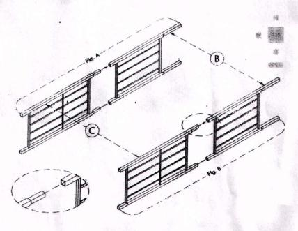
Now join the two Top Panels – A, push the female ends onto male ends as shown. When these are snug, insert bolts, add nuts and tighten with wrench.
